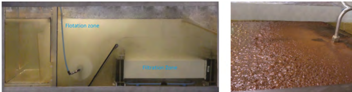
Figure 11.13.7. Side view of the akvoFloat pilot (left) and resulting float layer during operation (right).
