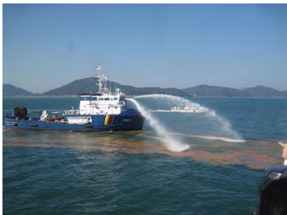
Figure 7.4. Clay dispersal for HAB control in Korea. Photo: D.M. Anderson.
