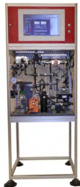
Figure 3.14. Components of a Ferrybox system: Left: sensors for conductivity, oxygen, chlorophyll fluorescence (proxy for phytoplankton biomass), phycocyanin fluorescence (proxy for cyanobacteria biomass), and turbidity Photos: Bengt Karlson; right: an example of a fully configured, commercially available Ferrybox system: http://www.4h-jena.de/ .
