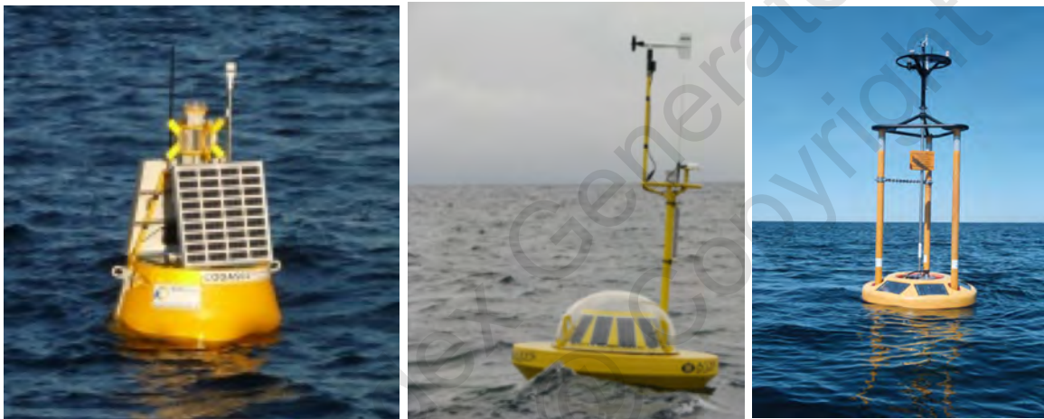
Figure 3.11. Examples of instrumented oceanographic buoys operated by the Swedish Meteorological and Hydrological Institute. The most important parts, i.e. the underwater sensors, are not shown. Left: the coastal Koster fjord buoy in the Skagerrak, Sweden designed by Techworks Marine Ltd. Ireland, middle: the offshore Huvudskär buoy in the Baltic Sea designed by Axys Technologies Inc. Canada, and right: the offshore Läsö buoy in the Kattegat, between Sweden and Denmark, designed by Fugro-Oceanor, Norway. Photos: Fredrik Waldh, Henrik Lindh/Per Olsson and Bengt Karlson.
